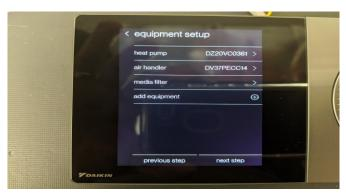
Step 4: Select "Heat Pump or AC" or select "Furnace or Air Handler" in order to access the menu folders for each unit. Otherwise, select "Next Step" to move to the next screen.
